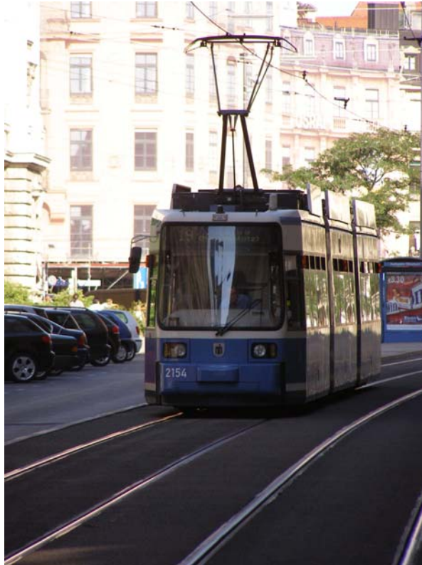
Tram: Runs on tracks through town or city. Notice the wires overhead. The wires supply electricity that runs the tram
